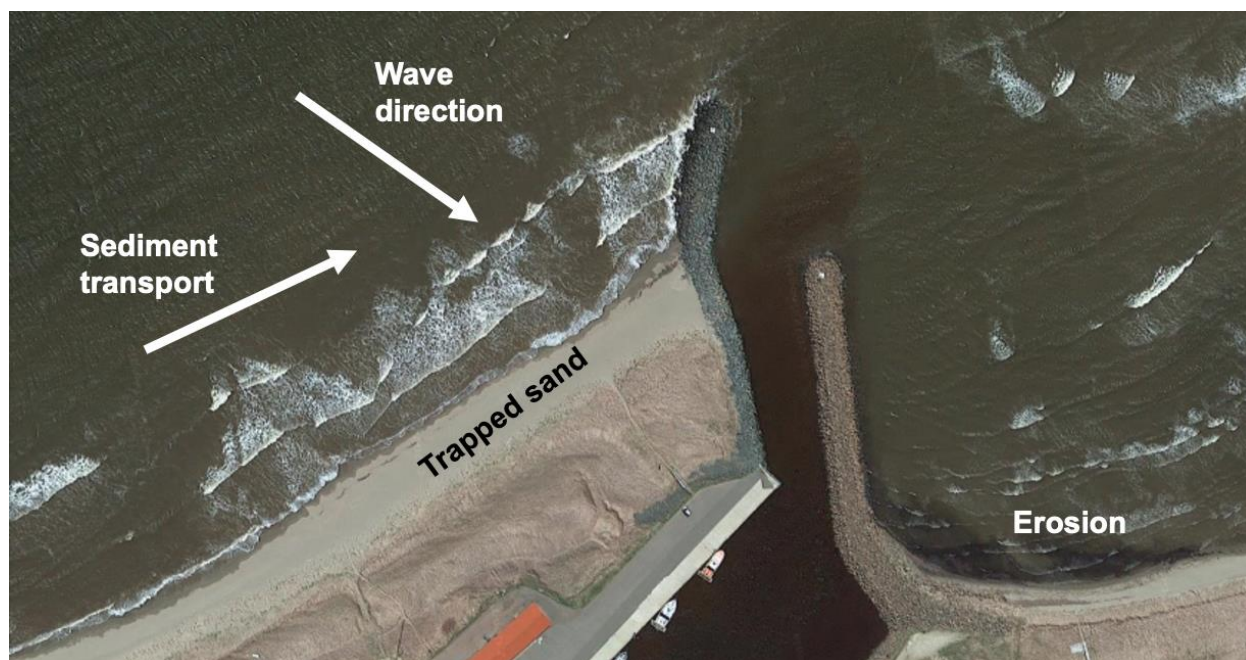
Figure 1.3 Accretion (trapped sand) and erosion at shore-perpendicular structures. Engineered structures can interfere with natural flow and sediment processes and may have unintended consequences further down the coast (Google Earth, 2022)
