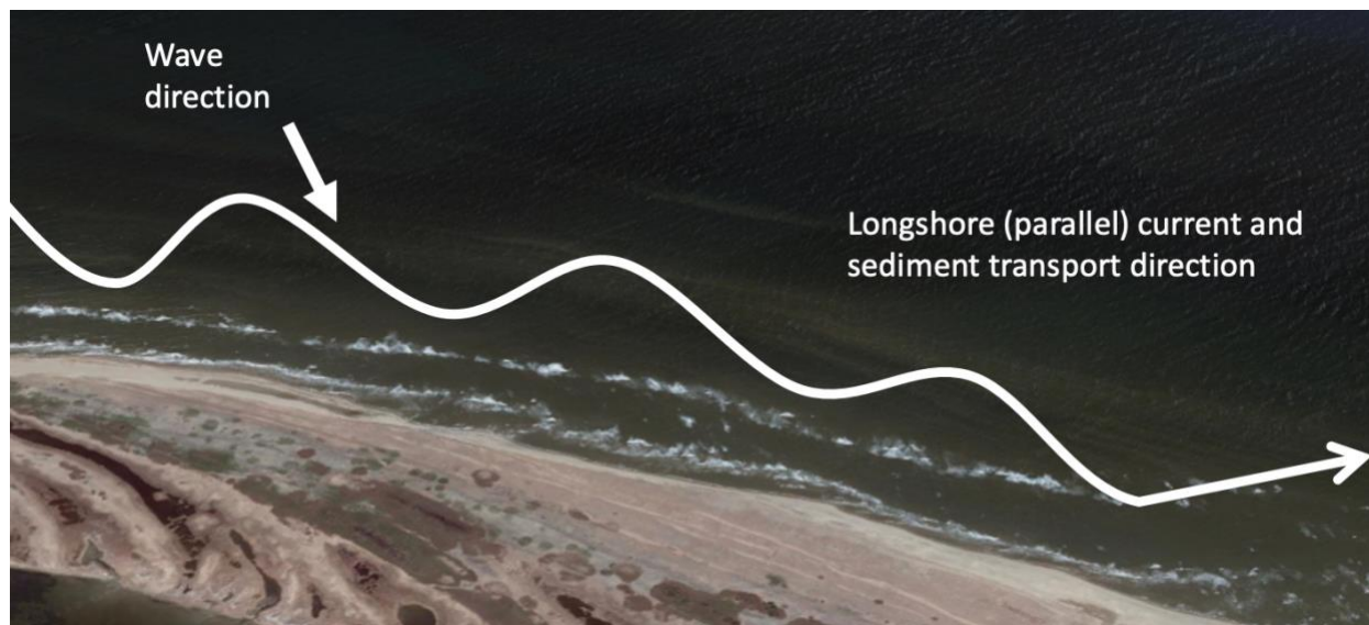
Figure 1.2 Illustration of longshore (parallel) sediment transport (modified from Google Earth 11 )
