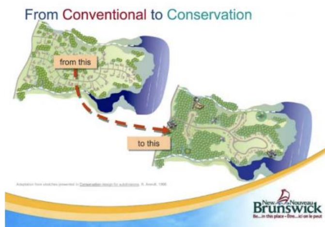
Figure 2.47 Example of site design differences between traditional subdivision design and conservation subdivision design (Daniel Savard, New Brunswick)
