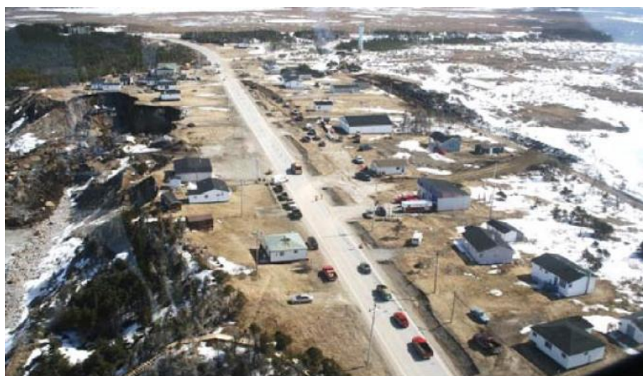
Figure 2.45 The Town of Daniel's Harbour after the landslide in 2007. The landslide area can be seen in the top left of the photo. The road was abandoned and houses to the left of the road were removed. The construction of a new road can be seen to the right of the houses (Government of Newfoundland and Labrador)
