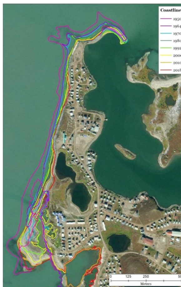
Figure 2.43 Aerial image of Tuktoyaktuk in 2010 showing the receding coastline between 1950 and 2018 (Future Tuktoyaktuk, images provided by NRCan 264 )
