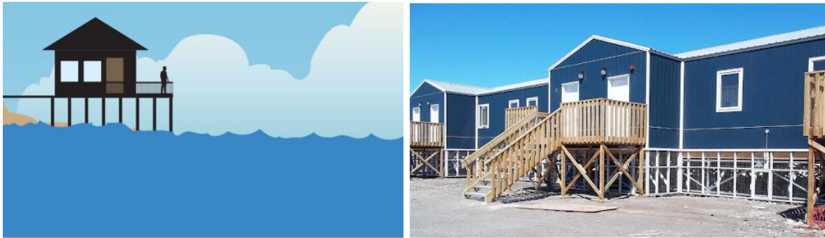
FIGURE 3. SCHEMATIC SHOWING WET FLOOD PROOFING AND AN EXAMPLE OF A MULTIPOINT FOUNDATION (TRIODETIC MULTIPOINT FOUNDATIONS). IMAGE SOURCE CLIMATLANTIC COASTAL ADAPTATION TOOL (2023)
